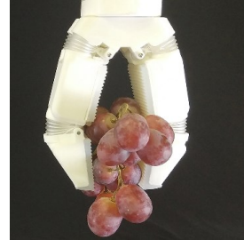
Figure.1. The 4-DOF compliant gripper Edgy-2.
