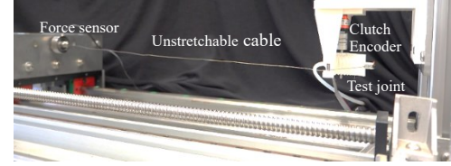
Figure.6. Joint test platform.
