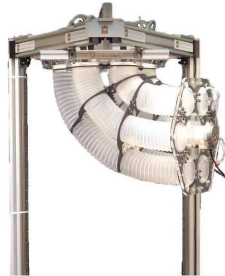
Fig. 2. The length of ExtenSA could reach from 100mm to 500mm, with a maximum elongation ratio of 400%. The bending angle of ExtenSA is  $100^\circ$ , and the payload of ExtenSA could reach more than 20kg vertically.
